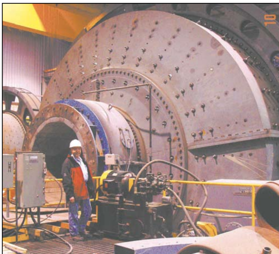
Heinz Drews of Invermere with the huge mill that rotates and crushes the ore.
